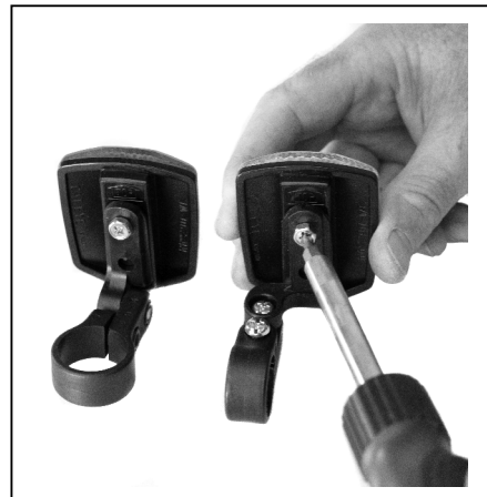
fitting the reflectors
