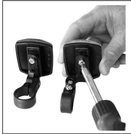
fitting the reflectors
